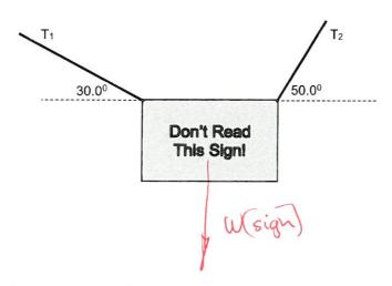
(a) Calculate the tensions  $T_1$  and  $T_2$  by use of a vector diagram.
