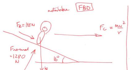
(b) Calculate the centripetal force acting on the motorbike.
